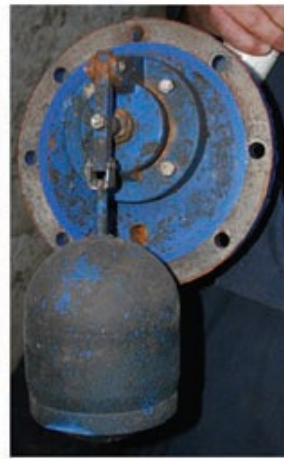
Fusion Bonded Epoxy (All After 3 years)
