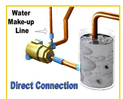
In this example the pressure created by the pump may be greater than the pressure in the make-up line. Thus, the make-up line is subject to backpressure. This is a direct cross-connection.
