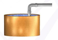
A <u>low inlet</u> is a direct cross-connection if the supply line is subject to backpressure. If the incoming line can not be subjected to backpressure it is not a direct crossconnection, but an indirect cross-connection.
